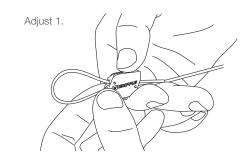
Ensure a minimum 75 mm of tail wire exit the hanger.
