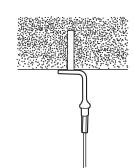
Position eyelet over drilled hole
